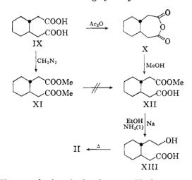
The synthesis of the lactone II from transcyclohexane-1,2-diacetic acid (IX)11 via its anhydride (X), acid ester (XII), and hydroxy acid
